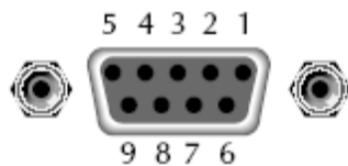
RS-232 connector pinout
