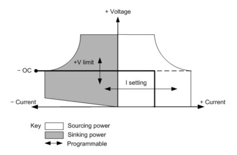
The heavy solid line illustrates the locus of possible operating points as a function of output. As shown by the vertical portion of the line, the output current remains regulated at its programmed setting as long as the output voltage remains within its limit setting. A CC (constant current) status flag indicates that the output current is being regulated and the output voltage is within its limit settings.
