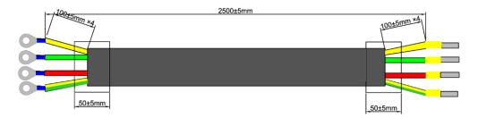
The red, green and yellow wires are live wires, which are correspondingly connected to the L1, L2 and L3 terminals of power input on the rear panel of the
