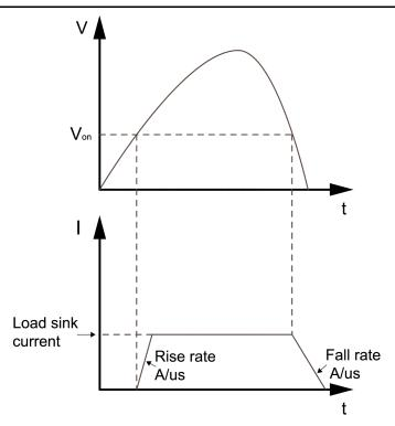
When VON LATCH function is started, the load starts load test only when the power voltage rises and is higher than Von Point loading voltage. When the power voltage drops and is lower than Von Point unloading voltage, the load will unload.
