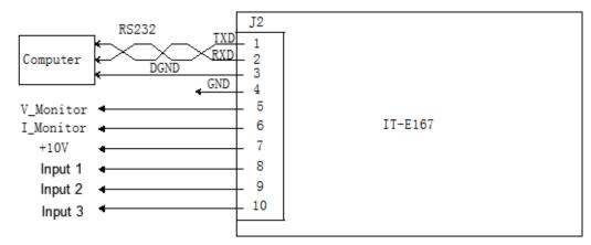
When using the RS-232 interface for communication, connect the pin 1, pin 2, and pin 3 of the IT-E167 to the PC. The pin description is as follows:
