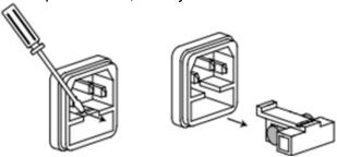
Replace with a fuse of the same specification and install it.
