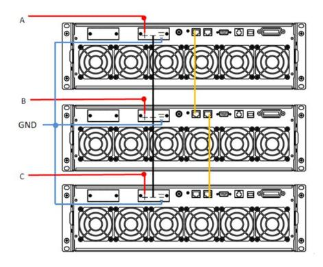
SYSTEM BUS: User need to connect three units together via a straight network cable. Please see figure above.
